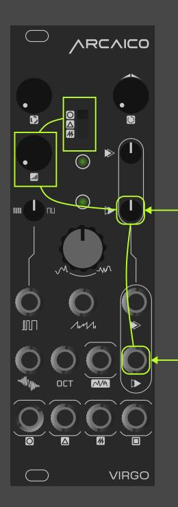
This is the CV attenuator, with this you can manage the amount of source control with a value between 0 (no control) to MAX.
